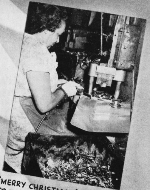
1. STAR SHAPES ARE BLANKED OUT OF THE METAL AT PRESS SUCH AS J.H. NORMANDIN OPERATES IN THE BLANKING ROOM.
