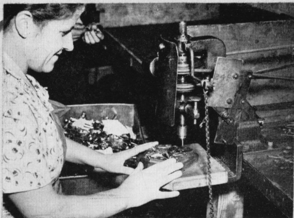
4. GIOVANNINA NANNI, ELECTRIC SHELL, TAPS THE BACKS OF THE ORNAMENTS FOR THE SCREWS WHICH WILL HOLD THE ORNAMENT TOGETHER.
